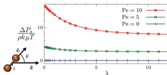
Fig. 5 Increase in bulk solvent pressure  $\Delta P_s$  as a function of the strength  $\lambda$  of the soft colloid–membrane interaction potential in the setting of Fig. 1 for active dumbbells at varying activity  $Pe$ . For active systems ( $Pe > 0$ ),  $\Delta P_s$  depends on  $\lambda$ .
