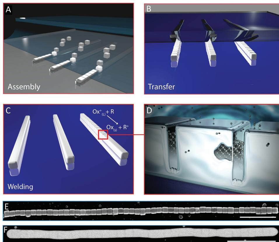
**Figure 1.** Diagram of the process presented. A) Direct assembly from solution of nanocubes into trenches patterned in a PDMS mold. B) Transfer of the assembled nanocubes to a new substrate. C) Epitaxial welding of the nanocubes into a patterned monocrystalline material via solution processing. D) Artistic representation of the epitaxial nanowelding process. E) SEM image of silver nanocubes on a silicon substrate before and F) after chemical welding. The scale bars are 500 nm.
