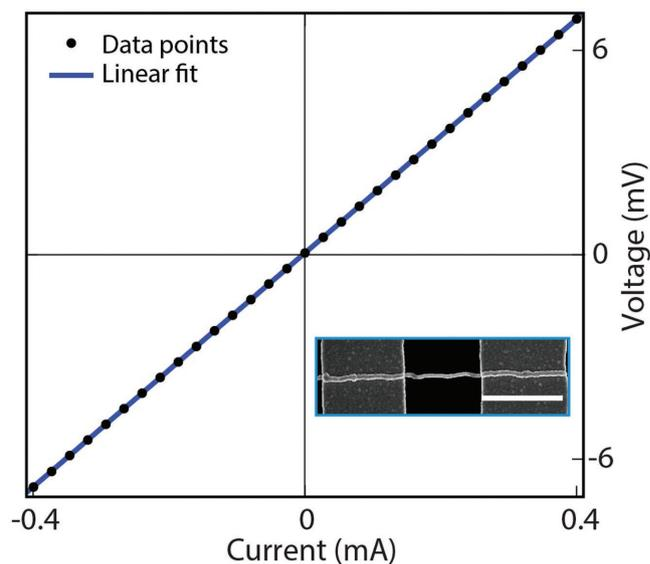
**Figure 4.** Electrical characterization of a 6  $\mu$ m long welded line. A resistance of  $R = 17$   $\Omega$  is measured, which corresponds to a resistivity of  $2 \times 10^{-8}$   $\Omega$ m. The inset shows an SEM image of the two internal contacts at which the voltage is measured. The scale bar is 2  $\mu$ m.
