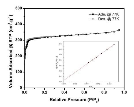
Surface area =  $1154 \text{ m}^2/\text{g}$ Slope = 3.013Intercept = 2.469e-03Correlation coefficient, r = 0.999954C constant = 1221Pore volume =  $0.50 \text{ cm}^3/\text{g}$  **Supplementary Figure 3.** Representative FE-SEM images of well-ordered superstructures self-assembled from ZIF particles of different sizes: a)  $178 \pm 8$  nm; b)  $193 \pm 8$  nm; and c)  $227 \pm 10$  nm. Scale bars: 5  $\mu$ m (left column) and 2  $\mu$ m (right column).
