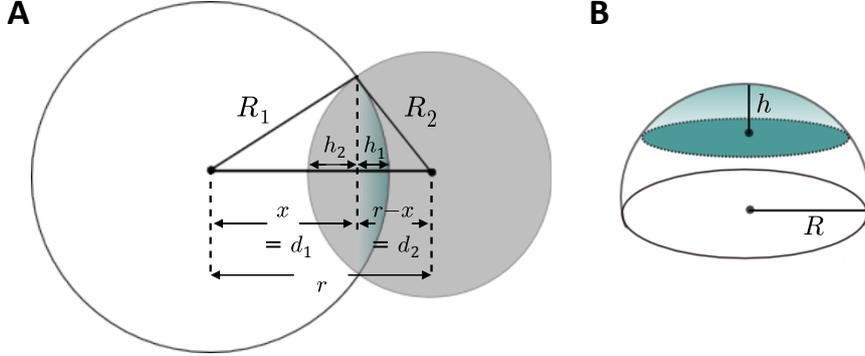
Figure S1: (A) Schematic representation of the overlap volume between two unequally sized spheres separated by a center-to-center distance  $r$ . The overlap volume is the sum of the volumes of two spherical caps with cap height  $h_1$  and  $h_2$ , where  $h_{1,2} = R_{1,2} - d_{1,2}$  and  $d_1 + d_2 = r$ . (B) A schematic representation of a hemisphere with radius  $R$  with a spherical cap with height  $h$  on top.
