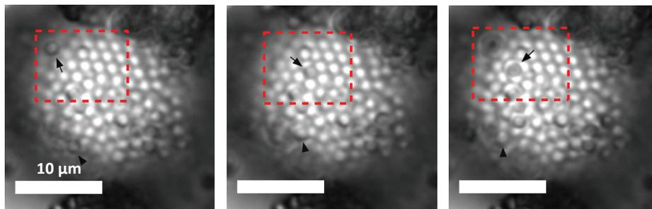
Figure S4: Small polystyrene particles attach and detach from a microsphere in time ( $\phi_d = 0.50$ ). The particle indicated by the black arrow inside the red box has an escape time of  $\tau = 127$  s. On top of the first layer of bound small spheres, multiple layers start to form. The triangle  $\blacktriangle$  indicates a small sphere that is hopping over the first layer of polystyrene particles. The scalebars represent  $10 \mu\text{m}$ .
