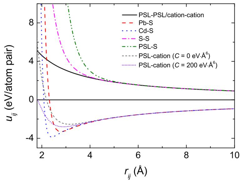
Supplementary Figure 1: **Interatomic pair potentials as a function of the interatomic distance  $r_{ij}$ .** The parameter  $C$  in the PSL-cation interatomic potentials is either 0 or 200  $\text{eV}\cdot\text{\AA}^6$ .
