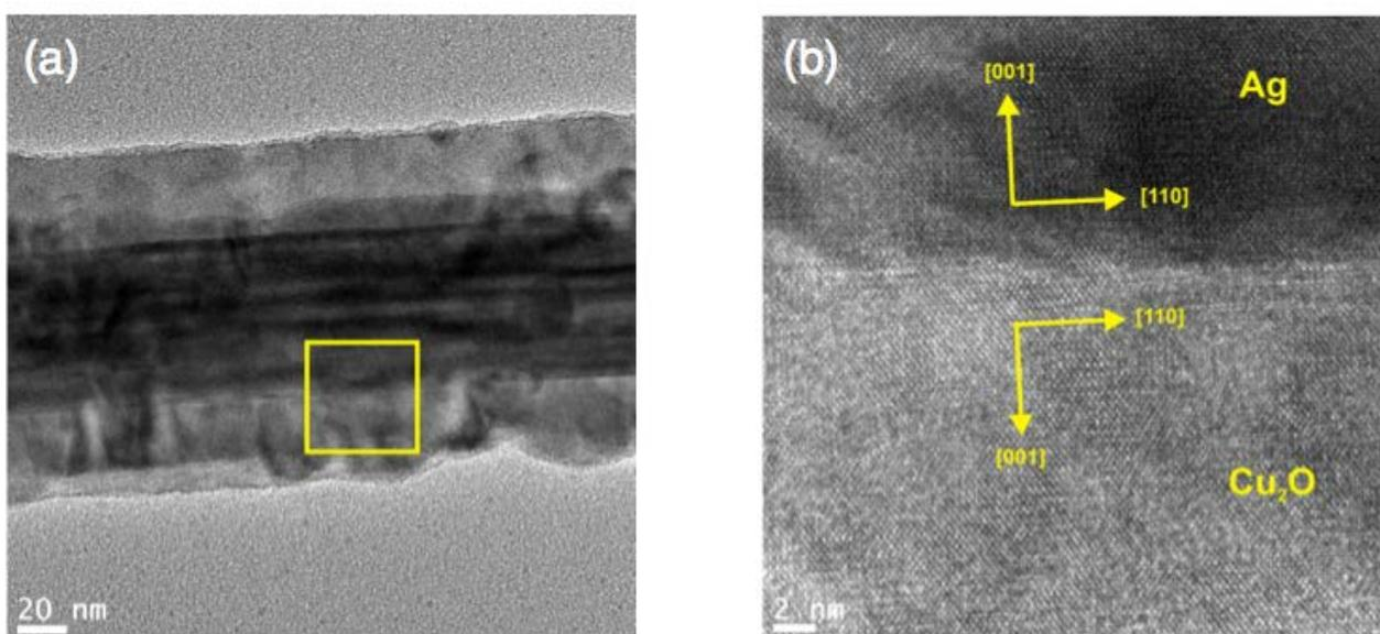
Fig. S6: (a) TEM image of Ag-Cu<sub>2</sub>O nanowires. (b) HRTEM of the Ag-Cu<sub>2</sub>O interface, with crystallographic directions.
