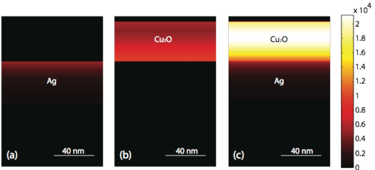
Fig. S2: Profile of the power absorbed in (a) a 100 nm Ag film, (b) a 40 nm Cu<sub>2</sub>O membrane and (c) a 40nm Cu<sub>2</sub>O membrane on a 100 nm Ag film. The power is weighted over the AM1.5 spectrum for photons above the band gap (290-650 nm). The color scale is in W/m<sup>2</sup> for a 1 V/m incident plane wave.
