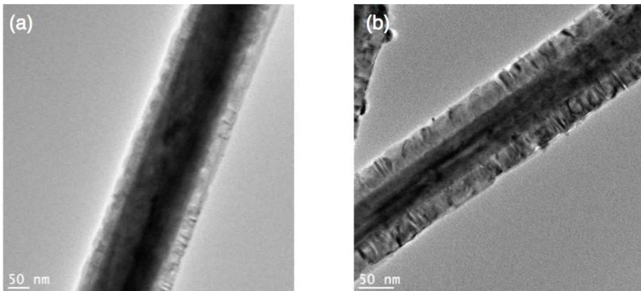
Fig. S5: (a,b) TEM images of Ag-Cu<sub>2</sub>O nanowires. The images show some low-angle planar defects (b), as well as parts with a long range purely monocrystalline Cu<sub>2</sub>O shell (a).
