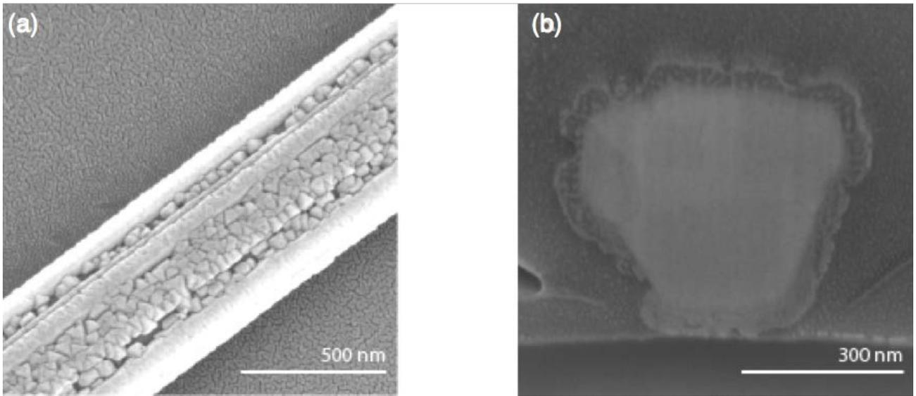
Fig. S3: (a) SE and FIB cross section of a Ag-Cu<sub>2</sub>O nanowire with a thick core.
