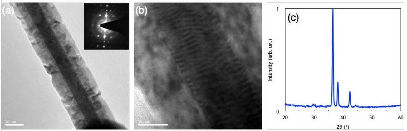
Fig. S1: (a,b) TEM image and (b) XRD of a Au-Cu<sub>2</sub>O NW. Moiré fringes are clearly visible in (b), indicating the crystallinity of the Cu<sub>2</sub>O shell.
