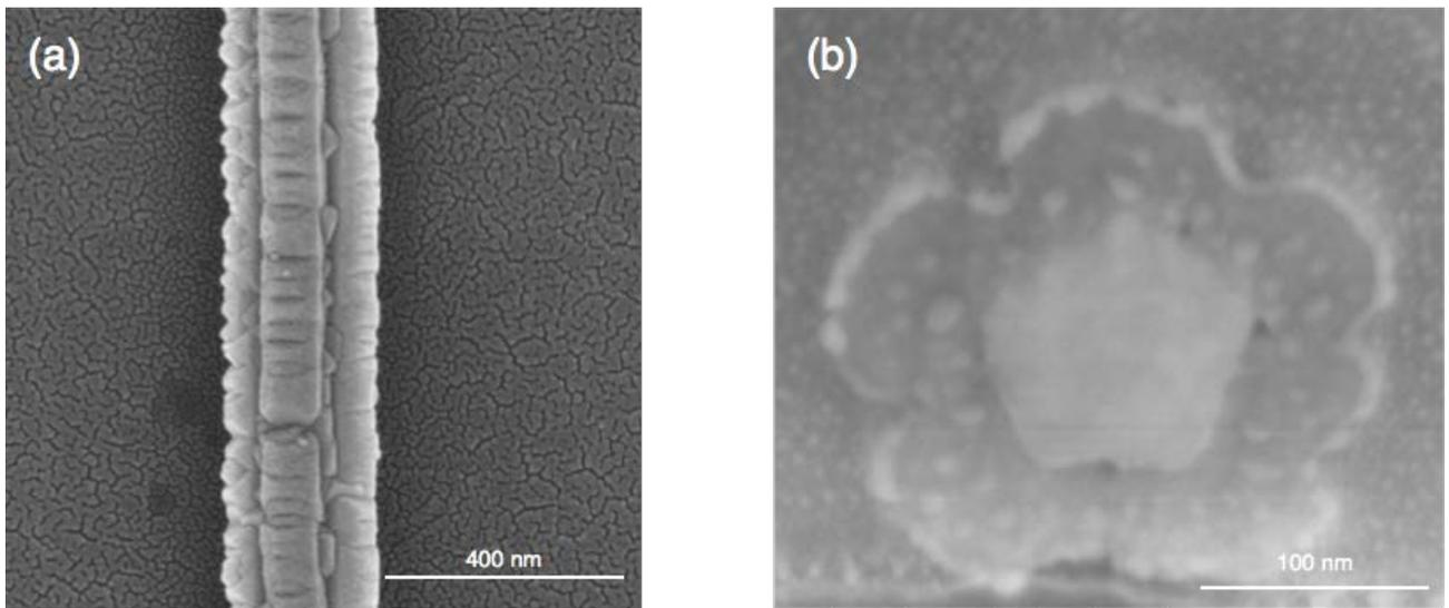
Fig. S4: SE (a) and FIB cross section (b) of the Ag-Cu<sub>2</sub>O nanowire measured in Fig. 3(a).
