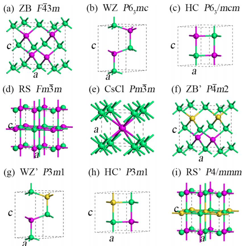
FIG. 1. Unit cells for binary compounds ((a)-(e)) and for QMPs ((f)-(i)). (a) ZB, (b) WZ, (c) HC, (d) RS, (e) CsCl, (f) ZB', (g) WZ', (h) HC', and (i) RS'. The space groups are listed for each structures. The green spheres represent one type of cations (Cd or Pb); yellow and purple spheres represent two different anions (S and Se).
