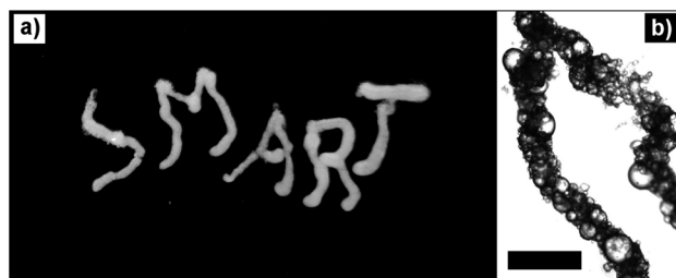
Fig. 7 (a) Photograph of concentrated emulsion (prepared at 60 wt% oil and stabilized using a 1 : 1 w/w mixture of XG : SL) extruded using a syringe and a needle in an acidic medium and (b) microscopy image of the extruded strand of emulsion droplets (scale bars = 400 \mu\text{m} ).
