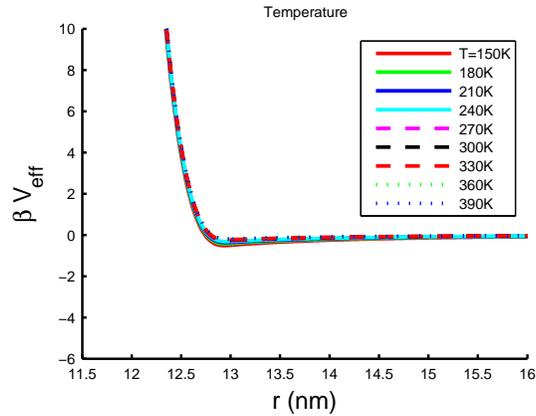
FIG. S9: Effective interactions between two 10 nm semiconductor nanoparticles for temperatures as labelled and with Hamaker constant  $A = 0.3$  eV, capping layer thickness  $L = 1.5$  nm, and ligand distance  $s = 0.43$  nm.
