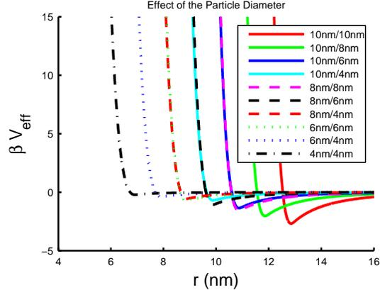
FIG. S7: Effective interactions between two gold nanoparticles for particle diameters as labelled with Hamaker constant  $A = 3$  eV, capping layer thickness  $L = 1.5$  nm, and ligand distance  $s = 0.43$  nm at room temperature ( $T = 300$  K).
