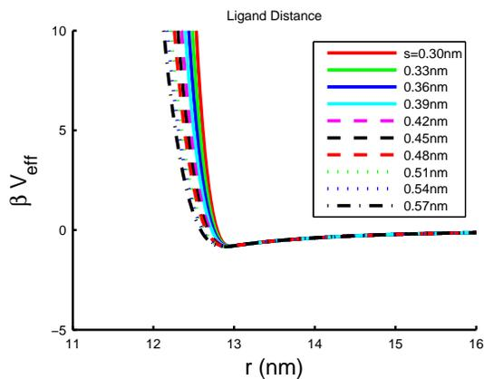
FIG. S17: Effective interactions between a 10 nm semiconductor nanoparticle and a 10 nm gold nanoparticle for capping layer densities  $s$  as labelled with Hamaker constant  $A = \sqrt{3} * 0.3$  eV, and capping layer thickness  $L = 1.5$  nm at temperature  $T = 300$  K.
