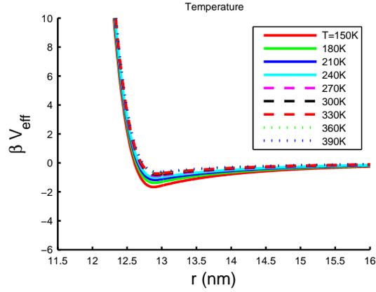
FIG. S11: Effective interactions between a semiconductor and a gold nanoparticle both with diameter 10 nm for temperatures as labelled and with Hamaker constant  $A = \sqrt{0.3 * 3}$  eV, capping layer thickness  $L = 1.5$  nm, and ligand distance  $s = 0.43$  nm.
