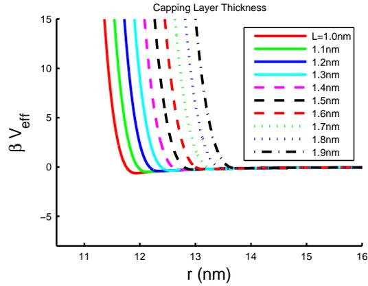
FIG. S12: Effective interactions between two 10 nm semiconductor nanoparticles for capping layer thicknesses  $L$  as labelled and with Hamaker constant  $A = 0.3$  eV, and ligand distance  $s = 0.43$  nm at temperature  $T = 300$  K.
