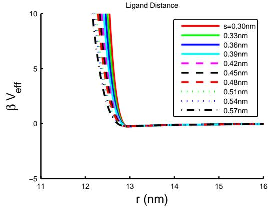
FIG. S15: Effective interactions between two 10 nm semiconductor nanoparticles for capping layer densities  $s$  as labelled with Hamaker constant  $A = 0.3$  eV, and capping layer thickness  $L = 1.5$  nm at temperature  $T = 300$  K.
