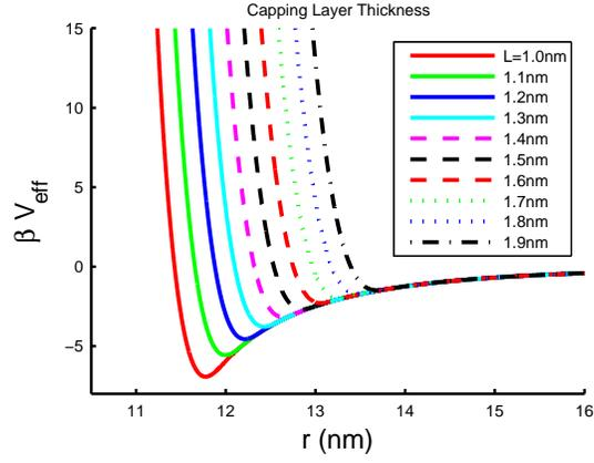
FIG. S13: Effective interactions between two 10 nm gold nanoparticles for capping layer thicknesses  $L$  as labelled and with Hamaker constant  $A = 3$  eV, and ligand distance  $s = 0.43$  nm at temperature  $T = 300$  K.
