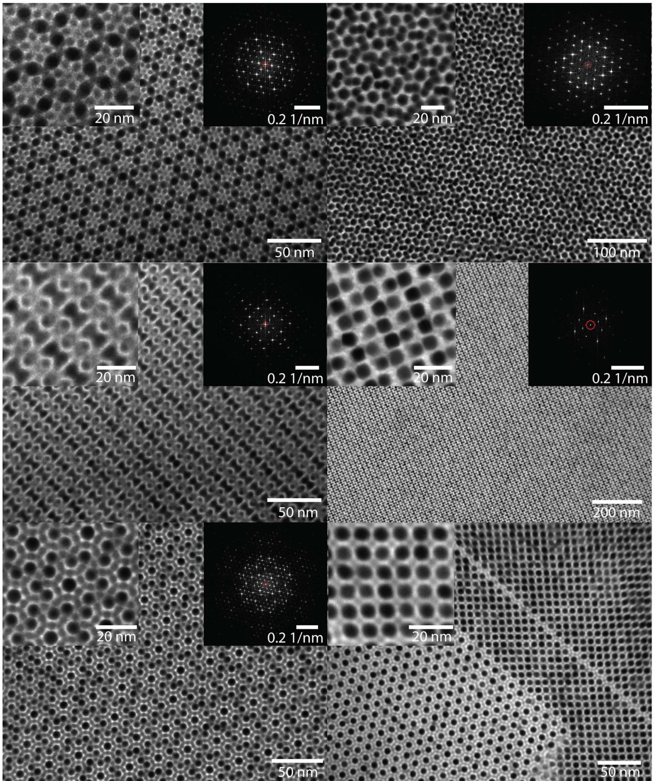
FIG. S3: Unknown binary superlattices obtained from PbSe and CdSe NCs at a size ratio  $\gamma$  between 0.60-0.63. In the inset of each of the images, a zoom in of the TEM pictures of the crystal structure and a Fourier transform are presented.
