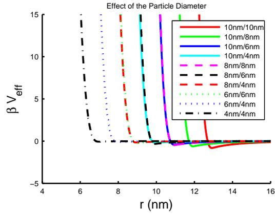
FIG. S8: Effective interaction between a semiconductor and a gold nanoparticle for particle diameters as labelled and with Hamaker constant  $A = \sqrt{0.3 * 3.0}$  eV, capping layer thickness  $L = 1.5$  nm, and ligand distance  $s = 0.43$  nm at temperature  $T = 300$  K.
