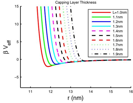
FIG. S14: Effective interactions between a 10 nm semiconductor nanoparticle and a 10 nm gold nanoparticle for capping layer thicknesses  $L$  as labelled with Hamaker constant  $A = \sqrt{3} * 0.3$  eV, and ligand distance  $s = 0.43$  nm at temperature  $T = 300$  K.
