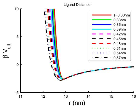
FIG. S16: Effective interactions between two 10 nm gold nanoparticles for capping layer densities  $s$  as labelled with Hamaker constant  $A = 3$  eV, and capping layer thickness  $L = 1.5$  nm at temperature  $T = 300$  K
