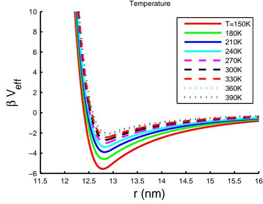
FIG. S10: Effective interactions between two 10 nm gold nanoparticles for temperatures as labelled with Hamaker constant  $A = 3$  eV, capping layer thickness  $L = 1.5$  nm, and ligand distance  $s = 0.43$  nm.
