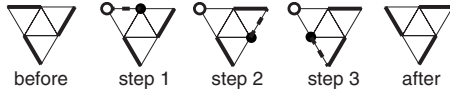
FIG. 9. An example of the bond switch move on a hexagonal lattice. The dumbbells are denoted by thick lines, the loose spheres by circles: \mathbf{r}(0) is shown by the open circle and the loose end, \mathbf{r}(1) is shown by the filled symbol. The bond configuration is depicted at the instant just after the bond indicated by a dashed line has been disconnected and before a new bond is chosen.
