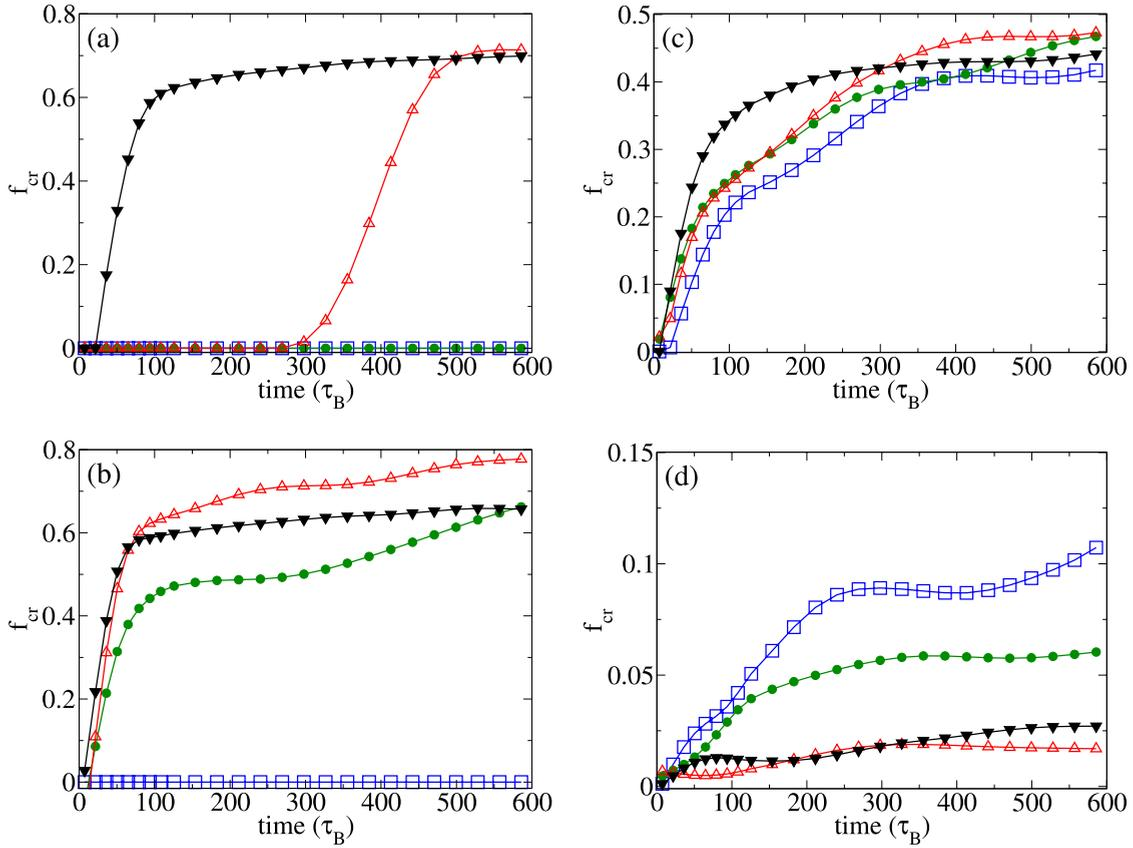
FIG. 7. (Color online) Crystal fraction  $f_{cr}$  as a function of time  $t$  for (a)  $\beta U=3.3$  (line A in Fig. 3), (b)  $\beta U=3.52$  (line in B Fig. 3), (c)  $\beta U=4.18$  (line in C in Fig. 3), (d)  $\beta U=6.6$  (line D Fig. 3). Squares indicate a colloid packing fraction  $\eta_c=0.05$ , circles indicate  $\eta_c=0.20$ , up triangles indicate  $\eta_c=0.40$ , and down triangles indicate  $\eta_c=0.45$  (same symbols as in Fig. 3).
