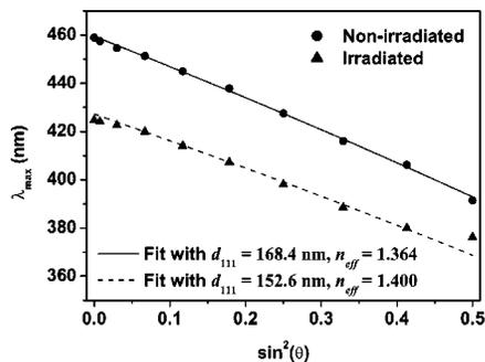
FIG. 4. Position of the transmission minima in Fig. 3 as a function of  $\sin^2(\theta)$ . After irradiation, the positions of the stop gap for ellipsoidal particles (triangles) shift to shorter wavelengths in comparison to the case of spherical particles (circles). The values are determined from the experimental spectra after correction for the background scattering. The lines are theoretical fits using  $\lambda_{\text{max}} = 2d_{111} \sqrt{\varepsilon_{\text{eff}} - \sin^2 \theta}$ .
