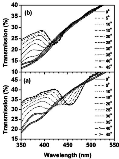
FIG. 3. Angle-resolved optical transmission spectra of colloidal photonic crystals of silica particles grown on a glass substrate. The spectra were taken from different points on the  $L \rightarrow W$  line towards the  $\Gamma$  point of the Brillouin zone. (a) Nonirradiated crystal of spherical particles. (b) Irradiated crystal of oblate ellipsoidal particles of aspect ratio  $1.65 \pm 0.09$ .
