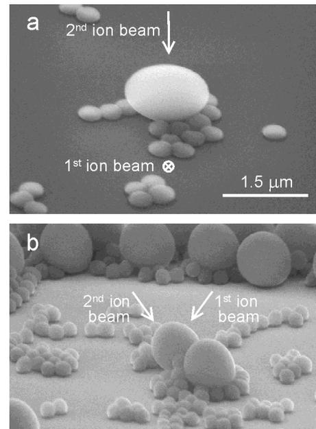
Fig. 3. Prolate ellipsoids: SEM images of silica particles such as those shown in Figure 1a–d, after an additional 4 MeV Xe<sup>4+</sup> ion irradiation to a fluence of  $3 \times 10^{14}$  cm<sup>-2</sup> at an angle orthogonal to the first irradiation. a) View along the direction of the first ion irradiation (+45° tilt). b) View almost perpendicular to the two ion beams (same orientation as in Fig. 1d).
