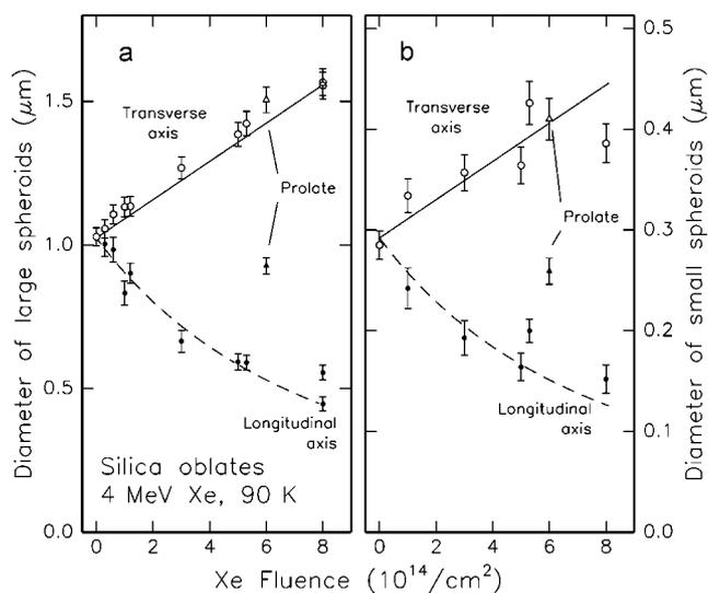
Fig. 2. Transverse and longitudinal diameters of a) large and b) small silica spheres as a function of 4 MeV Xe<sup>4+</sup> irradiation fluence. Circles correspond to oblate ellipsoids, and triangles to prolate ellipsoids made using two orthogonal irradiations. The line drawn through the data for the transverse axes is a linear fit, the dashed line is a calculation derived from the drawn line assuming the particle volume remains constant with fluence.
