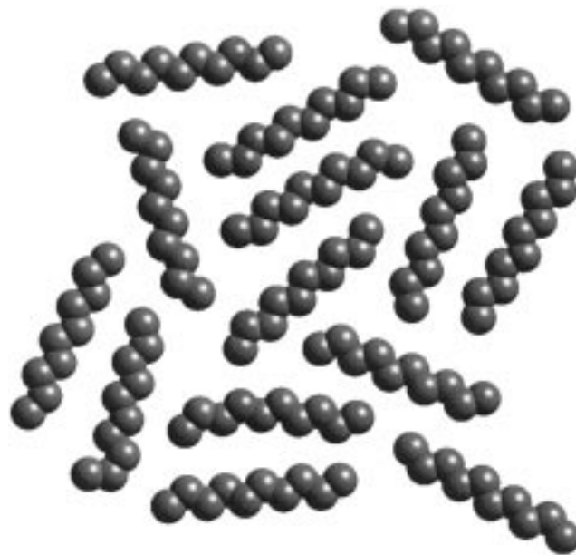
Fig. 4. Typical snapshot of n-decane ( xy -plane) at a plate separation of 5 \text{\AA} (top view).
