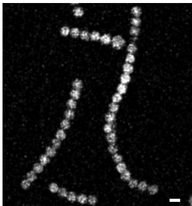
Figure 8.7: Confocal microscopy image of RITC labeled fluorescent emulsion droplet strings. Scale bar 5 \mu\text{m} .
