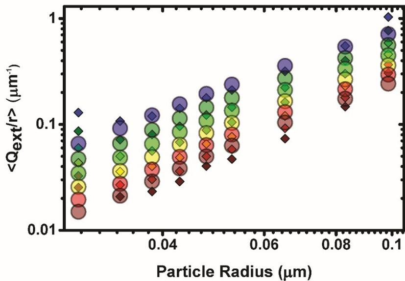
Figure S7:  $\langle Q_{ext}/r \rangle$  versus average particle radius measured on dilute samples (small squares) and calculated from Mie theory (large circles). Input for the theory is: a particle refractive index of 1.50, a particle density of  $1.1 \text{ g cm}^{-3}$ , and the measured particle volume distribution from DLS for each sample. Data are shown for six wavelengths, shown in colors from blue to red: 450, 500, 550, 600, 650, 700 nm.
