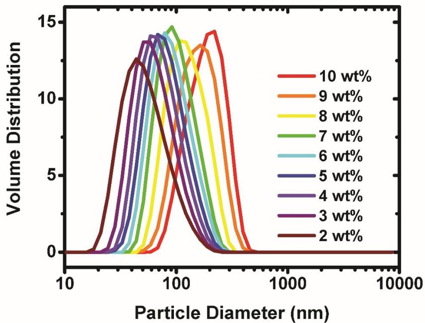
Figure S5: Size distribution data (volume distribution) for particles synthesized with varying wt% zein in the stock solutions. Data was taken from dynamic light scattering
