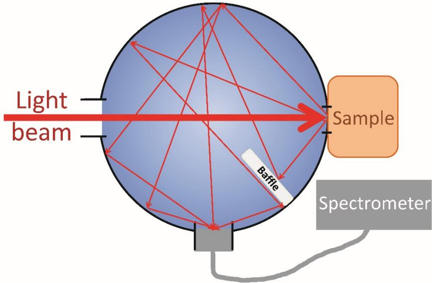
Figure S1: Schematic overview of the setup for total reflection measurements. An Integrating sphere of 15 cm in diameter was used (Labsphere). The sample opening was 12 mm, the detector port opening was 3 mm and the opening for the light beam was 6 mm.
