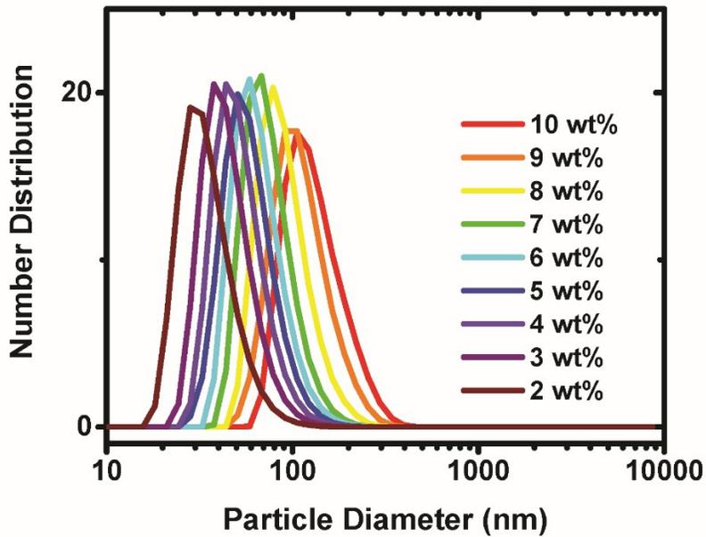
Figure S4: Size distribution data (number distribution) for particles synthesized with varying wt% zein in the stock solutions. Data was taken from Dynamic Light Scattering.
