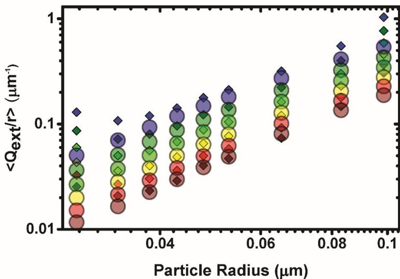
Figure S6:  $\langle Q_{ext}/r \rangle$  versus average particle radius measured on dilute samples (small squares) and calculated from Mie theory (large circles). Input for the theory is: a particle refractive index of 1.48, a particle density of  $1.1 \text{ g cm}^{-3}$ , and the measured particle volume distribution from DLS for each sample. Data are shown for six wavelengths, shown in colors from blue to red: 450, 500, 550, 600, 650, 700 nm.
