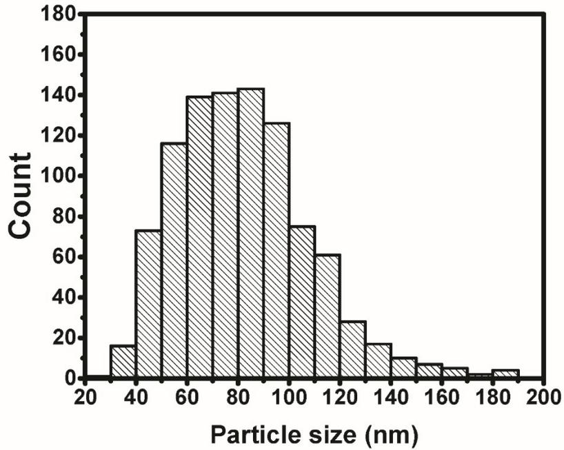
Figure S3: Manually counted particle sizes (diameters) from SEM images of the sample shown in Figure 2b, 960 particles were measured. This sample was synthesized from an 8wt% stock solution.
