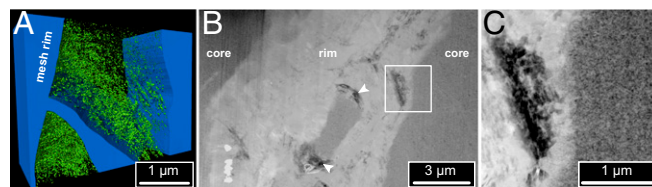
Fig. 4. Porosity within an organic-bearing, mesh-textured serpentinite clast. (A) Three-dimensional visualization of a FIB-SEM nanotomography volume ( 14.8 \times 11.05 \times 5.3 \mu\text{m} ) showing that mesh cores consist of an extensive network of aligned mesopores (green), whereas the rims (blue) are mainly characterized by individual micrometer-sized pores (arrowheads) as shown in HAADF-STEM image (B). (C) HAADF-STEM image of the interface between the mesh rim and the core (white rectangle in B). Note the pore size difference between mesh rim and core and the complex contrast in the core indicating nanoscale pore connectivity.
