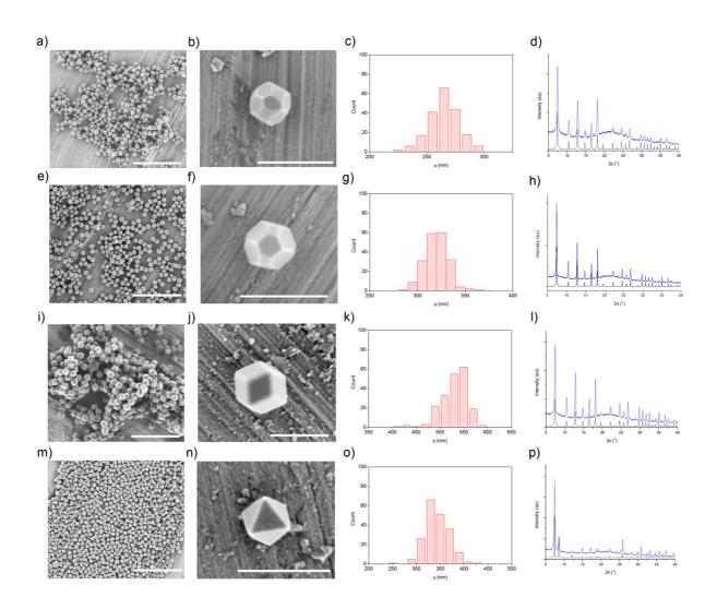
**Supplementary Figure 18.** Additional FE-SEM images of the self-assembled superstructures made of (a,b) TRD ZIF-8 particles with t = 0.57; (c,d) TRD ZIF-8 particles with t = 0.38; and (i,f) octahedral UiO-66 particles. Scale bars: 10 µm (c), 3 µm (a,e), 2 µm (b), and 1 µm (d,f).
