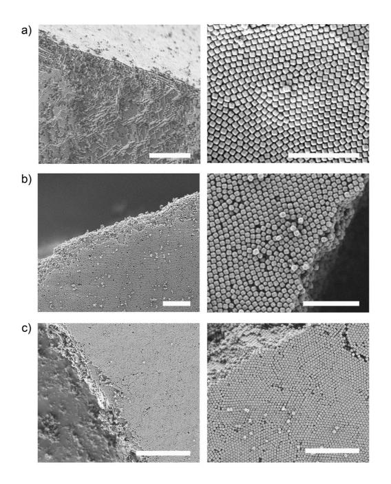
**Supplementary Figure 4.** Representative FE-SEM images of the self-assembled superstructures obtained using different techniques: a) evaporation at RT; b) evaporation at 100  $^{\circ}$ C; c) spin coating; d) dip coating; and e) vertical deposition. Scale bars: 10 µm (left column) and 5 µm (right column).
