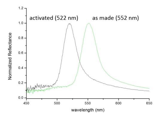
**Supplementary Figure 13.** Optical reflectance at  $\theta = 0^{\circ}$  for the photonic crystal made of TRD ZIF-8 particles sized 210 ± 10 nm: as-made (light green), activated (black), and after exposure of the latter to MeOH (red), EtOH (blue), *i*-PrOH (violet), or *n*-BuOH (dark green).
