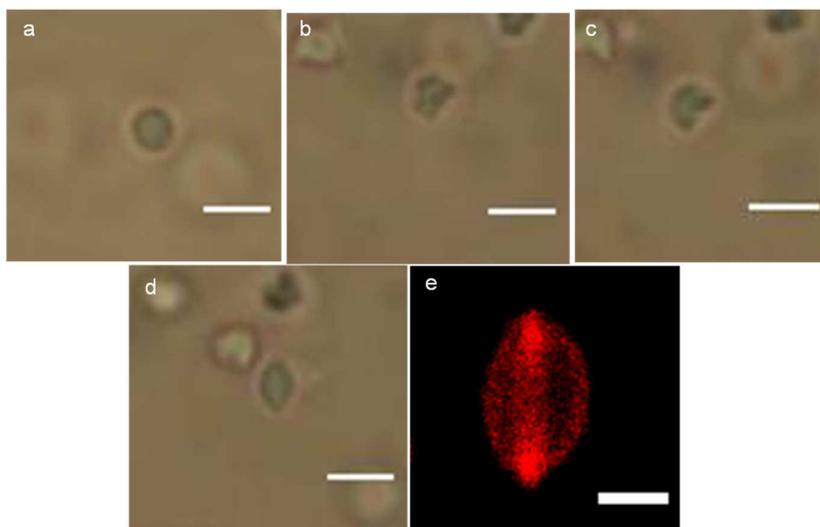
**Figure S1.** Optical microscope images of the morphology of extremely thin microcapsules,  $d/R_t < 0.005$  during the release of oil at (a)  $t = 0$  sec, (b)  $t = 120$  sec, (c)  $t = 125$  sec and, (d)  $t = 163$  sec. (e) Confocal picture of a coffee bean particle. All scale bars represent  $2\mu\text{m}$ .
