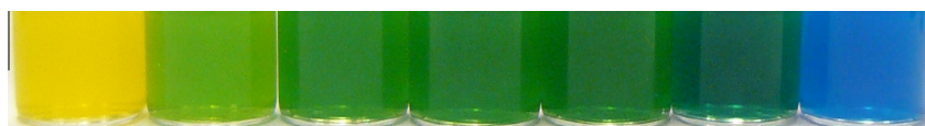
Fig. 1. Colloidal dispersions with a tuneable yellow–green–blue colour containing (from left to right) zein:Cur:IC (20:1:0; 20:1:0.25; 20:1:0.5; 20:1:1; 20:0.5:1; 20:0.25:1 and 20:0:1). The ratios are expressed on weight basis and the total concentration of zein in all cases was 1 wt.%.
