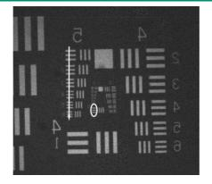
A two-photon 3D optical storage system based on a photochromic diarylethene (1,2-bis(2-methylbenzo[b]thiophen-3-yl)hexafluorocyclopentene) and a highly efficient two-photon absorbing fluorescent dye (2,7-bis[4-(9,9-didecylfluoren-2-yl)vinyl]phenylbenzothiazole) is demonstrated. The figure shows twophoton fluorescent readout of data recorded by single-photon excitation. The system is suitable for recording data in thick storage media and providing a non-destructive readout method.
