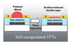
**Surface-induced phase separation** in polymer blends is used to fabricate self-encapsulated thin-film transistors. The semiconductor material preferentially wets the gate dielectric surface and a self-organized bilayer of two polymers phases occurs spontaneously (see figure). The encapsulant and semiconductor are deposited in one step.
