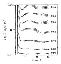
Fig. 1. – Velocity autocorrelation function multiplied by  $t^2$  in a four-dimensional lattice gas. The functions are shown for different densities f, defined as the average number of particle per link. Note that in all cases we observe the expected  $t^{-2}$  long-time decay.
