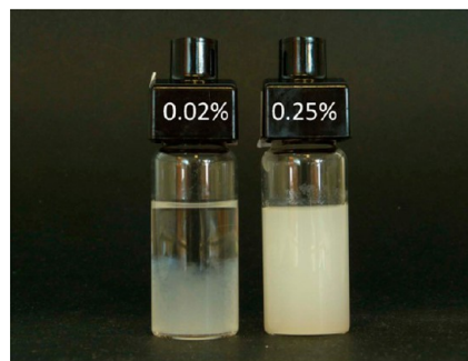
Figure 5. CMF dispersions ( N = 1 ) that form a collapsed gel at a concentration of 0.02% and a space-filling network at a concentration of 0.25% for a sample height of 4.0 cm.
