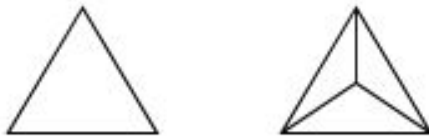
Figure 6: Subdivision of a single simplex (left) into subsimplices (right). A vertex is inserted into the single simplex and this vertex is connected by edges to the vertices of the simplex.
